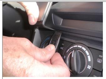
2. Press the thin end of the enclosed gap opener into the gap between the two dashboard sections, to widen the gap. Then press forwar on the lower part of the ProClip so the angled edge hooks into the gap next to the gap opener. Pull out the gap opener.
