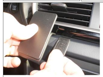
1. Press the thin end of the enclosed gap opener into the gap between the padded ledge in the dashboard and the trim below the air vent, to widen the gap.
